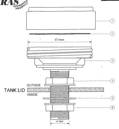
Install Connector onto Tank Lid by assembling Parts 3, 4, 5 & 6 in positions indicated.
