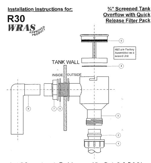
Install Connector onto Tank by assembling Parts 3, 6, 7 & 8 in positions indicated.
