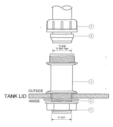
Install Connector onto Tank Lid by assembling Parts 1, 2 & 3 in positions indicated.
